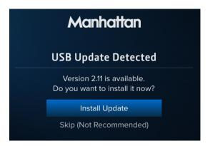
Connect the USB stick to the USB port on the box (see below) and wait few seconds for the USB Update Detected screen to be shown.
