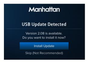
3. Connect the USB stick to the USB port on the box (see below) and wait few seconds for the USB Update Detected screen to be shown.
