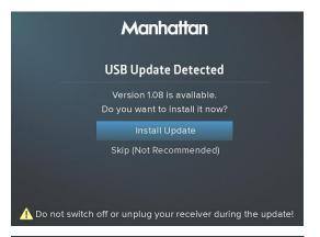
Connect the USB stick to the USB port on the box (see below) and wait few seconds for the USB Update Detected screen to be shown.
