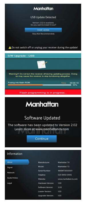
Connect the USB stick to the USB port on the back of the T3 and wait a few seconds for the USB Update Detected screen to be shown.
