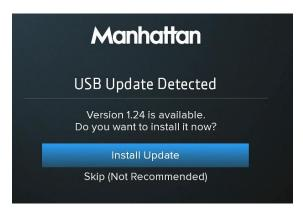
3. Connect the USB stick to the USB port on the back of the T3 and wait a few seconds for the USB Update Detected screen to be shown.
