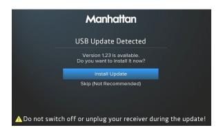
Connect the USB stick to the USB port on the back of the T3 and wait a few seconds for the USB Update Detected screen to be shown.
