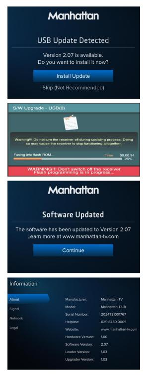
Connect the USB stick to the USB port on the back of the box and wait few seconds for the USB Update Detected screen to be shown.
