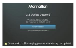
Connect the USB stick to the USB port on the back of the T3•R and wait a few seconds for the USB Update Detected screen to be shown.
