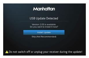
Connect the USB stick to the USB port on the back of the T3•R and wait a few seconds for the USB Update Detected screen to be shown.
