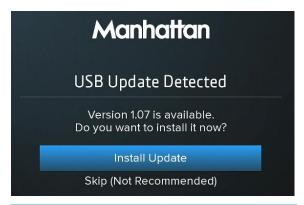
3. Connect the USB stick to the USB port on the back of the T3•R and wait a few seconds for the USB Update Detected screen to be shown.
