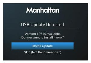
3. Connect the USB stick to the USB port on the back of the T3•R and wait a few seconds for the USB Update Detected screen to be shown.
