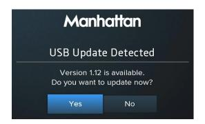
3. Connect the USB stick to the USB port on the back of the T2•R and wait a few seconds for the USB Update Detected screen to be shown.
