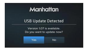
3. Connect the USB stick to the USB port on the back of the T2•R and wait a few seconds for the USB Update Detected screen to be shown.
