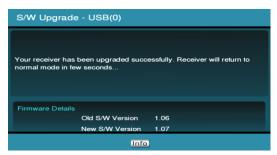
5. After the update is complete the Your receiver has been upgraded successfully screen will be briefly shown before the T2•R automatically reboots. The version will also be shown again after reboot. Check that it is 1.07.
