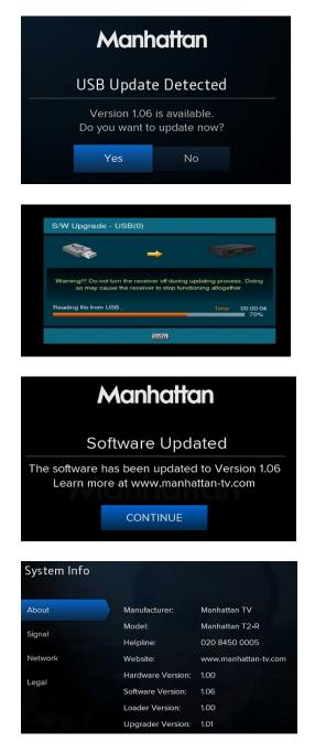
Connect the USB stick to the USB port on the back of the T2•R and wait a few seconds for the USB Update Detected screen to be shown.
