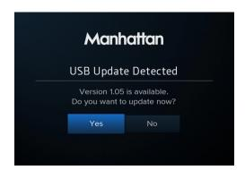
Connect the USB stick to the USB port on the back of the T2•R and wait a few seconds for the USB Update Detected screen to be shown.
