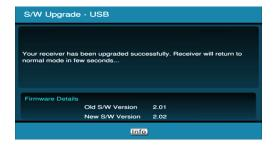
**5.** After the update is complete, the Your receiver has been upgraded successfully screen will be briefly shown before the T1 automatically reboots. The version will also be shown again after reboot. Check that it is 2.02.
