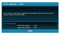
**5.** After the update is complete, the Your receiver has been upgraded successfully screen will be briefly shown before the SX automatically reboots. The version will also be shown again after reboot. Check that it is 1.04.
