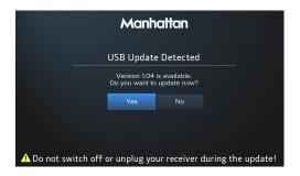
Connect the USB stick to the USB port on the left side of SX and wait a few seconds for the USB Update Detected screen to be shown.
