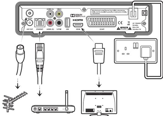
**To use Apps like BBC iPlayer or YouTube**, the Plaza HD•T2 must be connected to your internet router or hub using an ethernet cable (not supplied). Plug one end of the ethernet cable into the ETHERNET socket at the back of the Plaza HD•T2, and the other into your hub or router. Make sure the connections are fully pushed in - you'll hear a click as they lock into place. Consult your router or hub's documentation for further guidance.
